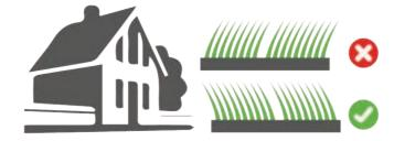
It is recommended to leave the grass to settle, before installing, for a minimum of 24 hours, to acclimatise and allow any creasing, wrinkling or pressure marks to fall out. This is due to it being flattened after being tightly rolled up in storage.
